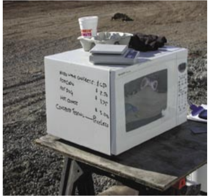
Fig. 2: Microwave unit for testing water content per AASHTO requirements
