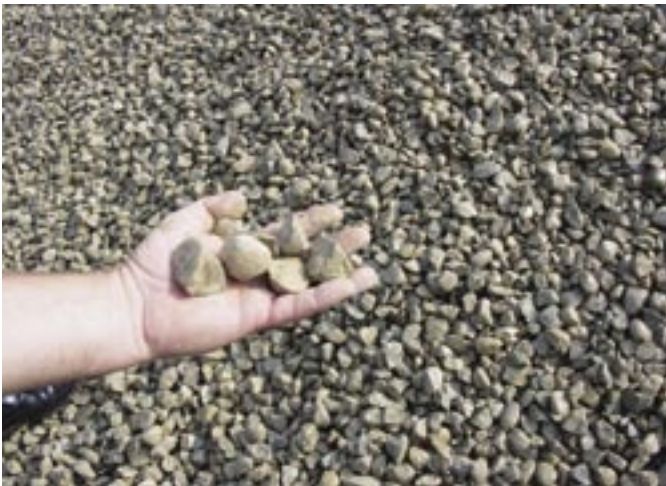
Fig. 3: Coarse aggregate used for the distribution center concrete (No. 467 stone [37.5 to 4.75 mm])
